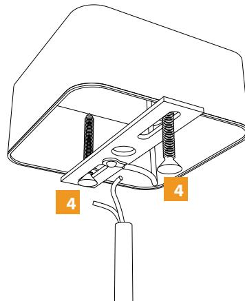
**2** Set strain relief at desired point on cord.
