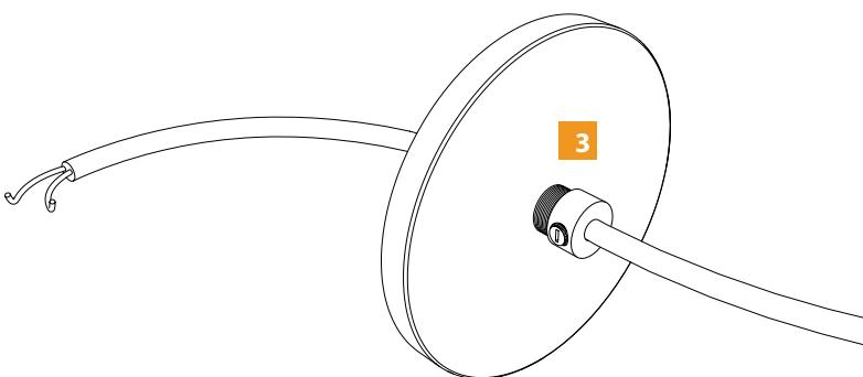
**6** Reassemble canopy to ceiling, turn the power on.
